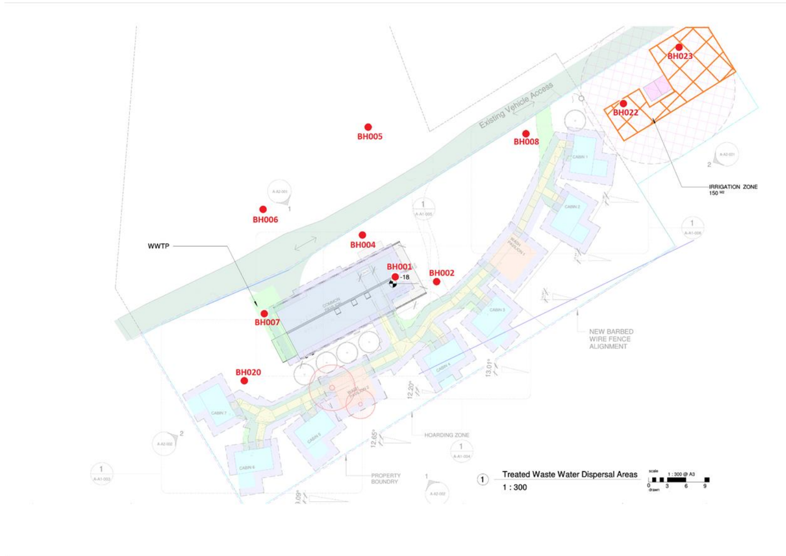
Figure 3 Layout of the Amphitheatre View EcoCamp showing location of infrastructure, the proposed treated wastewater irrigation field, and boreholes drilled for soil characterisation
